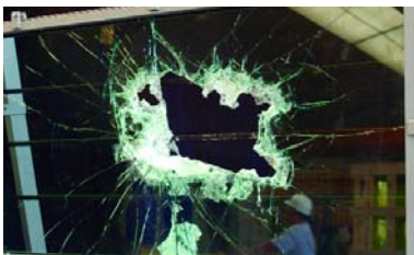
Conventional bulletproof glass. Has a large hole after 9 blows with a hammer.
