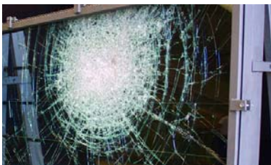
Crimaza Glass. Remains impenetrable after more than 60 blows with a sledgehammer
