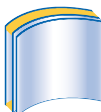
Double glazing with laminate on the inside
