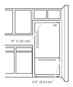
To ensure proper ventilation for your refrigerator, allow for 1/2" (1.25 cm) space at the top and behind the refrigerator for ease of installation.
