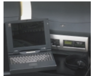
Technology interface panels may be mounted in the back of seats and with fold down tables offer exceptional utility even with laptops
