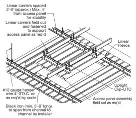
If the face of the access door rests slightly lower than the rest of the installation, fasten a metal shim to the top side of the grid where the 1-1/2" channel rests on it.
