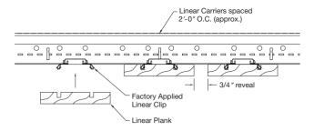
**CAUTION:** Be careful not to damage a clip. If a clip is damaged, a replacement clip can be put on from a spare piece of carrier.
