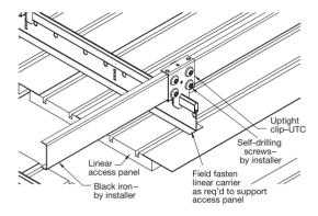
To create an access door in the field, first attach several field cut planks together with field cut carriers. Then use two pieces of 1-1/2" channel at least 3' long to act as outriggers to support the access panel. The channels should be attached at the bottom to the linear carriers with UTC clips. The weight of the access door will rest on the adjacent carriers.
