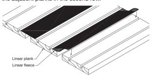
If there are any gaps between the fleece at plank end joints, cut a scrap of fleece from a leftover plank, apply a drop of glue to it and apply the patch over the gap on the back of the fleece.
