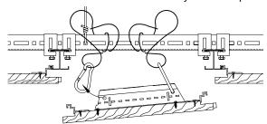
Step 5: Disconnect the panel safety cables.
