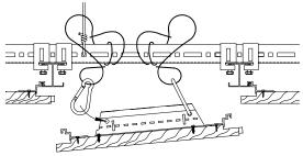
Step 1: Connect safety cables to WoodWorks panel.
