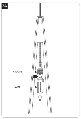
**CAUTION:** To reduce the risk of a burn or electric shock during relamping, disconnect the power to the fixture.
