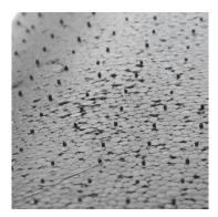
As a part of the production of EPP small raised dots will always be present on the surface. Expanding Polypropylene is recyclable and 100% non-toxic
