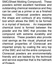
Clonecoat is Protech's line of powder coatings for the in-mold painting of
