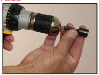
Insert drive socket (p/n 1993910) into a 0-2500 RPM screw gun.
