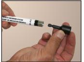
Insert Brick Tie drive socket into Condrive sleeve (3/16" Hex). Slide sleeve over drill adapter.
