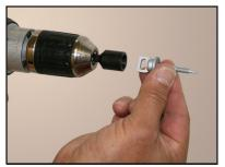
Insert Brick Tie Anchor into drive socket.
