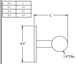
Pillar mounts to Junction box (by others) all junction boxes require suitable structural support mechanism such as blocking.
