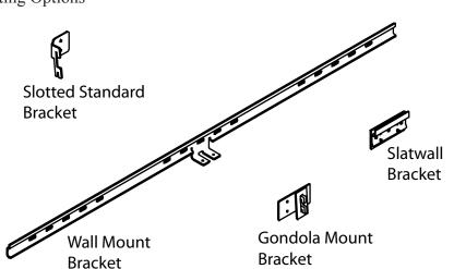
Mesa 4500 mounts directly to the wall, or with brackets mounts to slatwall, and slotted standards. All wiring connections to be installed by certified electricians according to local codes.
