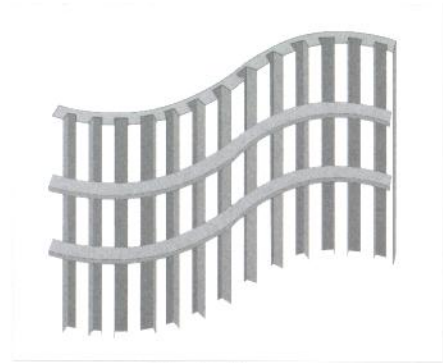
Single Layer Free Standing - Shaping Ribs
