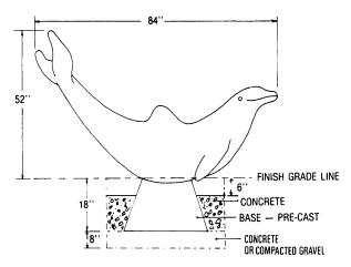
NOTE: THE PORPOISE MAY BE INSTALLED AT VARIOUS ELEVATIONS. THE LOWEST INSTALLATION POSITION IS SHOWN ABOVE.
