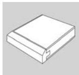
Veneer-Facet; solid wood T-edge on 1-1/8" particleboard (FA)
