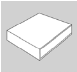
Laminate; 1-1/4" self edge; square corner (64E)
