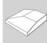
Veneer-Plateau; post-formed veneer over 1-1/8" MDF (PT)
