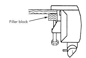
**NOTE:** If countertop is less than 1-1/2" (3.8 cm) thick, a filler block will have to be used for bolt to push against. (See figure 4)
