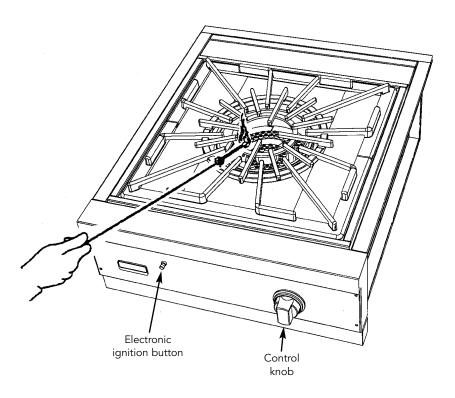
For proper lighting and efficient performance of the burner, it is necessary to keep the igniter and burner ports clean. If the flame is uneven, flutters, makes excessive noise or lifts, check to see if the burner ports are clogged. If the ports are clogged, use a wire, straightened paper clip, or needle to clear the ports. **Do not use a toothpick; it could break off in the port.** If the condition persists, contact an authorized service agency for adjustments.
