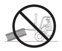
DO NOT lift Wood I Beam joists by top flange.
