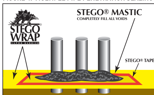
FIGURE 4: MULTIPLE PIPE PENETRATION SEALING
