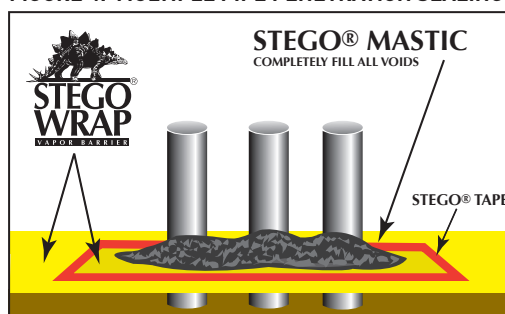
FIGURE 4: MULTIPLE PIPE PENETRATION SEALING
