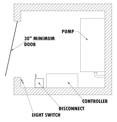
CONTOLLER MOUNTED ABOVE AND FLUSH WITH FRONT OF PUMP
