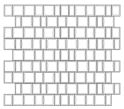
The Appian  $^{\!\scriptscriptstyle (\! R \!)}$  Mixed is manufactured to include three shapes: a nominal 6" x 6", 4" x 6" and 3" x 6". These bricks are to be laid randomly.
