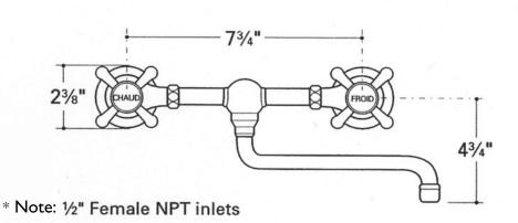
Spout projects 10" from wall Supplied with 11/4" European Lift & Turn drain with overflow
