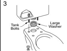
The tank should be inverted on the floor after removing the lid and parts bag. Open the plastic envelope and place the large doughnut shaped washer snugly on the threaded tank outlet. Invert the tank and lower onto bowl so that the large washer fits evenly into the bowl water inlet opening.
