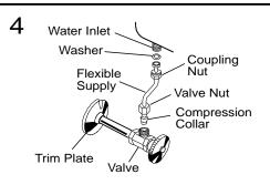
Connect the cold water line to the tank with your straight or angle stop. Place the washer, then the plastic nut on the tank end of the connecting pipe and bend the pipe to fit into the inlet hole on the water shutoff valve.
