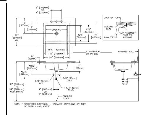
IMPORTANT: These dimensions are nominal and may vary within the range of tolerances established by ASME Standard A 112.19.2
