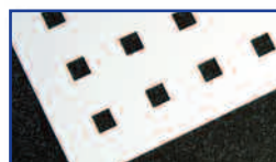
S14 Perforated Aluminum Pattern Shape: 1/4" square on 3/4" centers Open area: 11%
