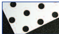
R38 Perforated Aluminum Pattern Shape: Round 3/8" x 1" staggered centers Open area: 13%
