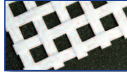
Basket Weave Perforated & Embossed Aluminum Pattern Shape: 7/16" square on 11/16" centers Open area: 34%
