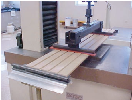
Panels During Load Testing
