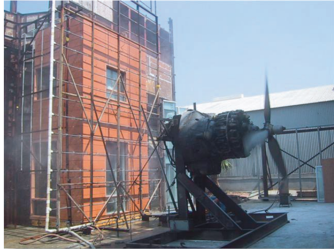
Rainscreen Panels in Place for Wind Driven Rain Testing
