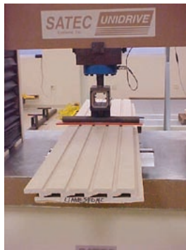
Panels During Load Testing
