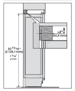
Cut a wooden beam (cross section min. 3" x 4" [75 mm x 100 mm]) to the required length.
