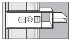
■ Do **not** remove the installation supports from the appliance door. They will be used later in the installation niche.
