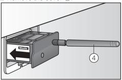
Push the module into the slot until it locks into place.
