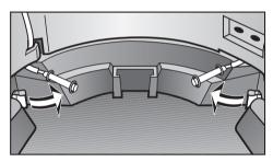
Unclip the water sensors and carefully bend them upwards.
