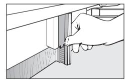
■ Wedge the air separator at the bottom of the freezer door, so it connects in place.
