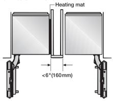
A heating mat must only be installed if the partition wall is less than 6" (160 mm) wide.
