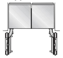
If the appliances are installed directly next to each other (without a partition), they need to be attached together using the "Merging Kit".
