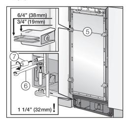
The installation aids (5) on the appliance door have been designed for custom door thicknesses of 3/4" (19 mm) and 1 1/2" (38 mm).
