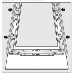
■ Insert the side strips all the way into the respective holes in the mounting frame.
