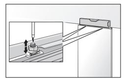
Align the custom door height with the double-threaded bolts.
