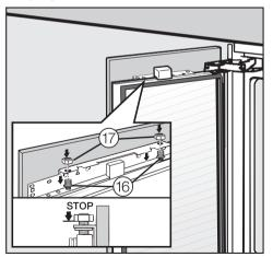
■ Open the upper door and hang the custom door with the adjusting rail over the double-threaded bolts (6).
