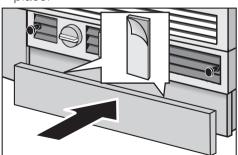
Remove the foil from the adhesive strips. Attach the toe-kick cover to the plinth.
