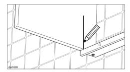
■ At the front edge of the spacer strip draw a vertical line on left and right side of the inside cabinet.
