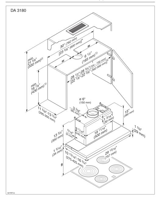
$<sup>^{\</sup>star}$  The hood can also be installed in a 23  $^{5}/_{8}^{"}$  (60 cm) cabinet.
