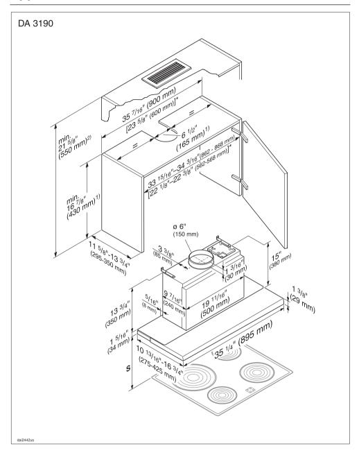
$<sup>^{*}</sup>$  The hood can also be installed in a 23  $^{5}/_{8}$ " (60 cm) cabinet.
