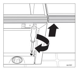
■ The deflector can be adjusted up to 2" (50 mm) towards the front with the two adjusting screws left and right in the deflector. Adjust the deflector until it is flush with the front of the adjacent cabinetry.
