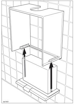
■ Insert the hood into the cabinet from below and until the spring clips click into place.
