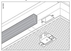
The installation kit DML 300 is necessary. It can be obtained as an optional accessory from Miele. The installation kit has an installation manual supplied.
