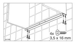
Screw the space bar flush with the wall under the cabinet side walls.
