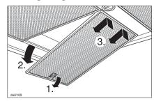
■ To remove the grease filter pull the locking clip forward. Lower the filter 45° unhook it at the rear and take it out. Support the grease filter so that it does not fall onto the cooktop.
