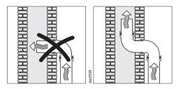
If the exhaust is ducted into an inactive flue, the air must be expelled parallel to the flow direction of the flue.
