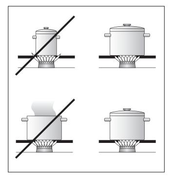
Pots with a diameter of less than **90 mm** or more than **280 mm / 320 mm for the large (WOK) burner** should not be used. When using large pots, pay attention to keeping to a minimum distance of **50 mm** between the cooking vessel and combustible surroundings.
