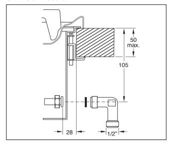
The gas connection must be in a location that permits access to the shut-off valve and which, if applicable, is visible after opening the door of the cabinet.
