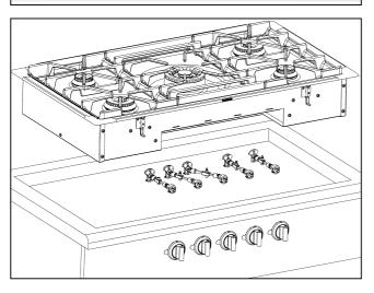
**Please note:** if you want to convert the appliance to a different type of gas, change the nozzles before installing the appliance (see pages 27-29).
