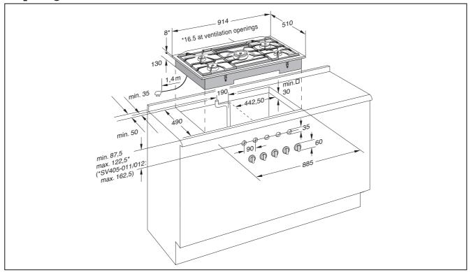
**Note:** the appliance can be installed in a base cabinet with a minimum width of 900 mm. The recess in the countertop will be slightly wider than the inner width of the base cabinet.
