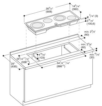
Immersion depth in the area of electric connection casing  $4^{13}/16^{"}(123)$
