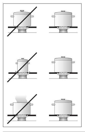
Pots with a diameter of less than **90 mm** or more than **280 mm** should not be used. When using large pots, pay attention to keeping to a minimum distance of **50 mm** between the cooking vessel and combustible surroundings.
