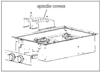
The numbers correspond to the diagram on the opposite page. Spindle extensions (SV 402-090 / SV 402-205) are available should the appliance be installed in a worktop which is non-standard depth.
