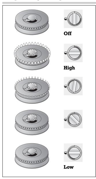
The appliance features one-hand operation, flame detection and automatic re-ignition. The ignition is activated when the control knob is turned.
