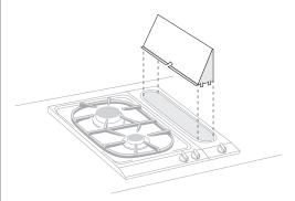
Place and snap the air baffle on the ventilation grill which has been turned over.
