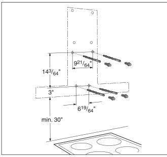
Remove the extractor hood. Drill the 4 lower 5/16" Ø fixing holes and press in the wall plugs flush with the wall..
