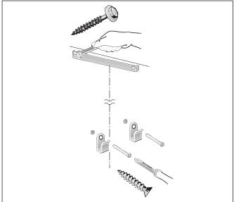
5 Screw on the upper and the two lower fixing brackets.
