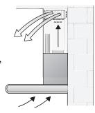
With activated carbon filter if exhaust-air mode is not possible.
