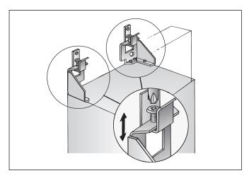
6 Attach the extractor hood. Adjust the height and align horizontally with the adjusting screws.
