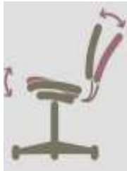
Seat Tilt Lock and Free Float
