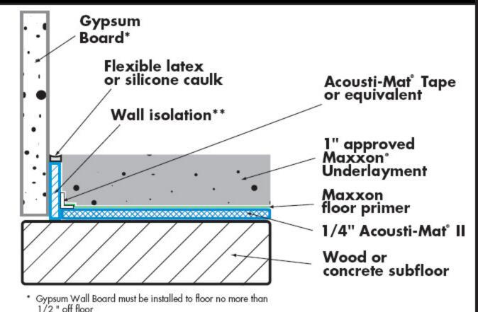
\*\* Wall Isolation is installed around the perimeter of the entire room to receive Acousti-Mat II, and around any floor penetrations such as toilet collars, electrical, plumbing, etc.
