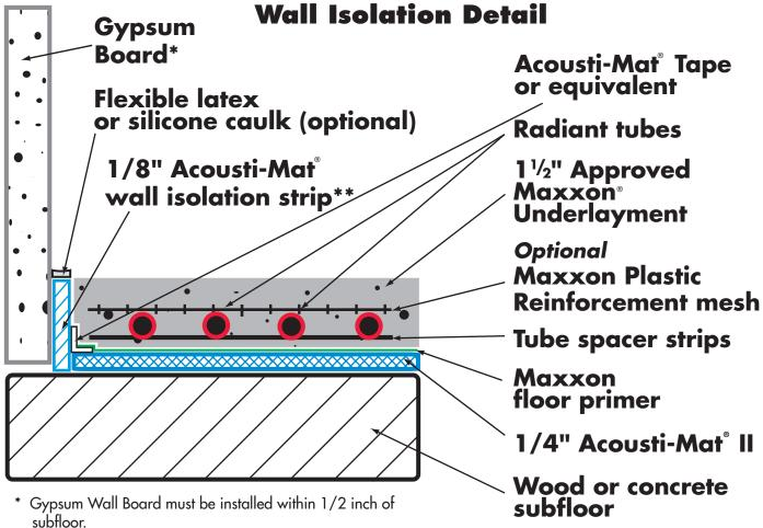
\*\* Acousti-Mat® Wall Isolation is installed around the perimeter of the entire room to receive Acousti-Mat II, and around any floor penetrations such as toilet collars, electrical, plumbing, etc.
