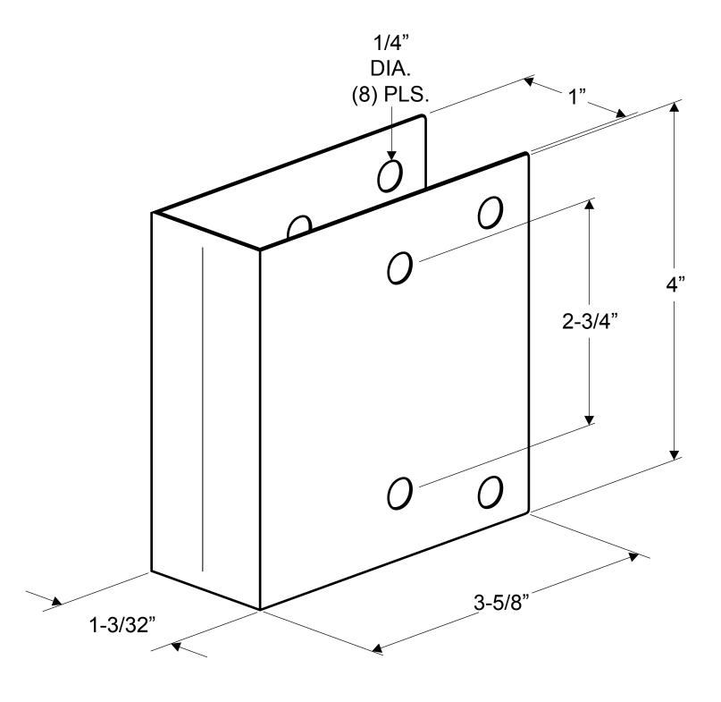
NOTE: PLATE FOR 115490, 115500, AND 115510 FIX-IT KITS WITH FASTENERS
