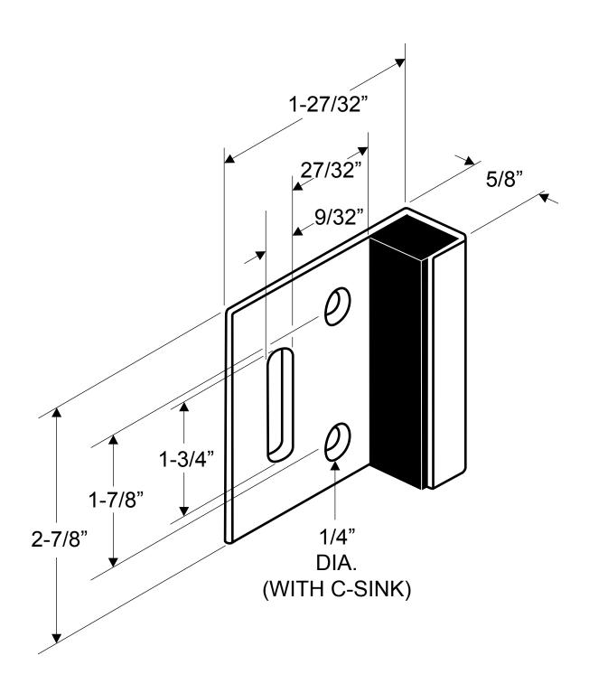
NOTE: FLAT-BACKED FOR WALL MOUNTING. 14 GAUGE (.075" THICK STAINLESS)
