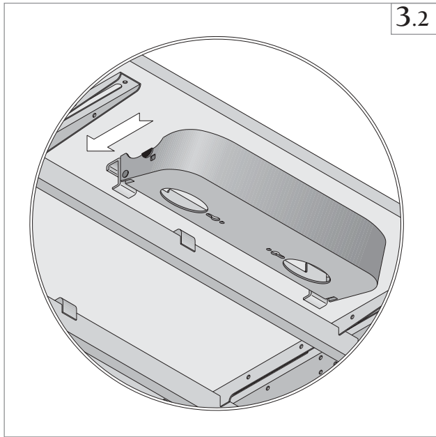
Snap electrical E-Box onto top frame.
