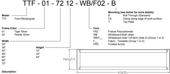
The frame is constructed using aluminum extrusion.
