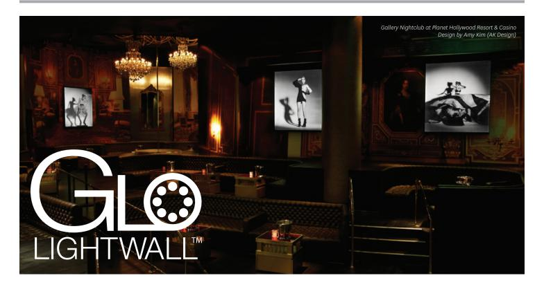
Pulp Studio's Glo Lightwall is a unified lighting panel which contains LEDs in itself as a source of light unlike the traditional back light units which are made by putting a lamp on the outside of acrylic sheet.
