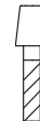
V Add $40 In-Set Pivot For mounting into horizontal surfaces. Requires a hole 0.65" in diameter
