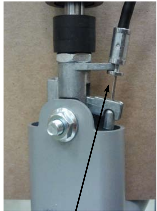
Slide in place.
