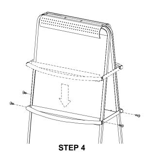
Slide tray support assembly over the top of unit with holes in round tube facing down and attach with the 1/4-20 x 7/8" Allen head screws. Tighten with Allen wrench provided.
